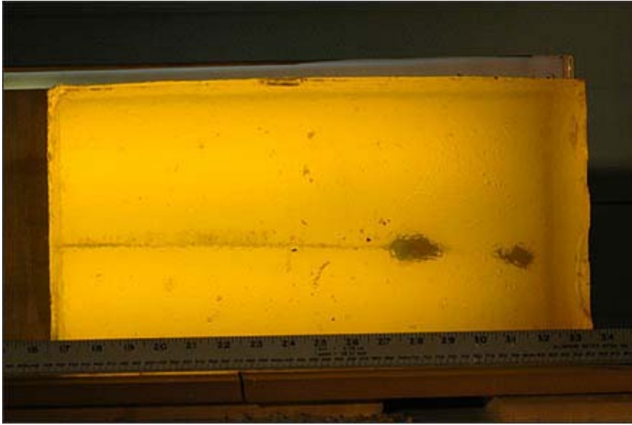
The second gelatin block showing the slug and wad material.
