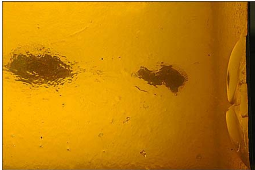
The second gelatin block showing the slug and wad material.
